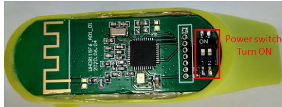
Fig4: Power switch Turn ON
